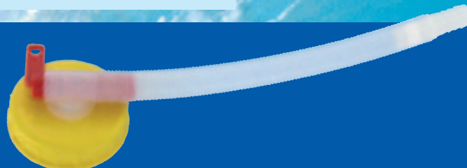
Screw cap DIN 96 with vented outlet valve Ø 20 mm and flexible hose 300 mm with barbed hosetail 20 mm (Hose length also on customer requirements) Article code 8072.82.10
