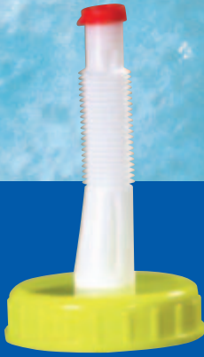
Pourer MINI DIN 96 with closing cap screwed into cap DIN 96 Front diam.: 22 mm, Length: 145 mm. Screwable from both sides of the cap Article code 8073.82.00
