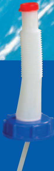
Pourer MINI DIN 51 with closing cap screwed into cap DIN 51 Front diam.: 22 mm, Length: 145 mm. Screwable from both sides of the cap. Article code 8273.01.00
